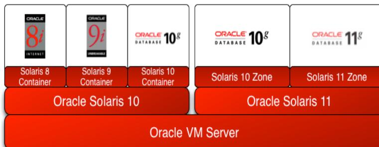
This diagram shows how four generations of OS can run in a virtualized system.
