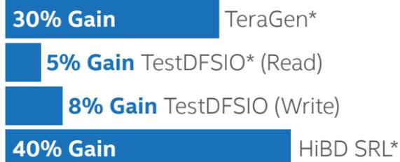
Figure 1. Benchmark test performance gains achieved after replacing the Ext4\* file system with the XFS\* file system
