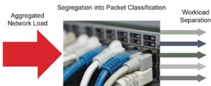
Figure 13. Packet classification in the ASIC's 10 Gigabit Ethernet Networking Technology enables network packets to be worked on in parallel.
