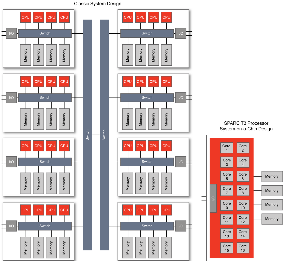
Figure 4. With 16 cores providing 128 threads, the SPARC T3 processor maximizes compute power and minimizes system component count at the same time, delivering greater reliability than systems with many more processors, multiple system boards, and far more complicated designs.
