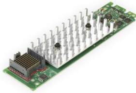
Figure 8. The Sun Dual 10GbE PCIe 2.0 FEM provides two 10GbE interfaces.
