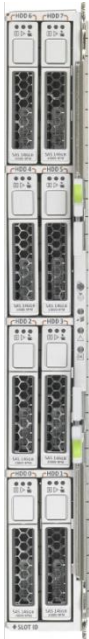
Figure 11. The Sun Blade Storage Module M2 provides up to eight SAS-2 drives which may be shared with other server modules within the Sun Blade 6000 chassis.
