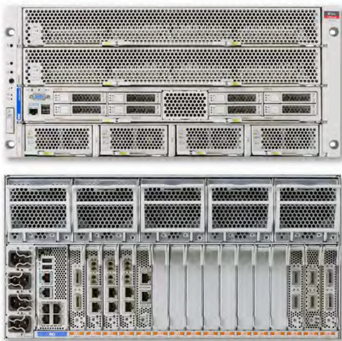
Figure 15. The front and rear panels of Oracle's SPARC T3-4 server.
