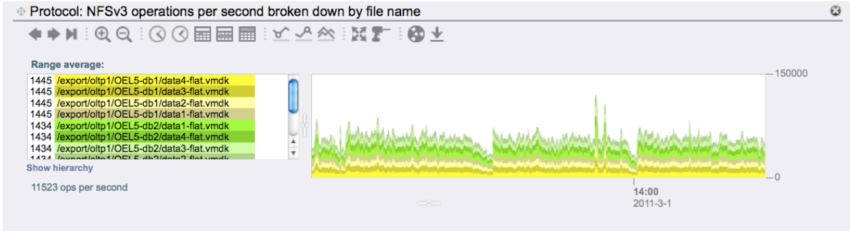
Figure 11. DTrace Analytics graph showing the number of NFS operations per second for the OLTP database virtual disks.
