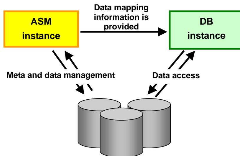
DB instance performs actual access to data files by using the data mapping information from the ASM instance.
