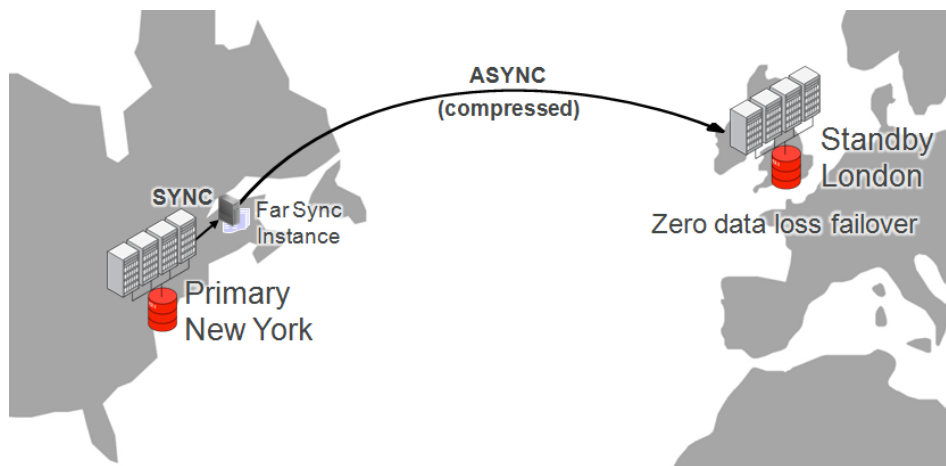
Figure 3: Active Data Guard Far Sync – Zero Data Loss Failover at Any Distance
