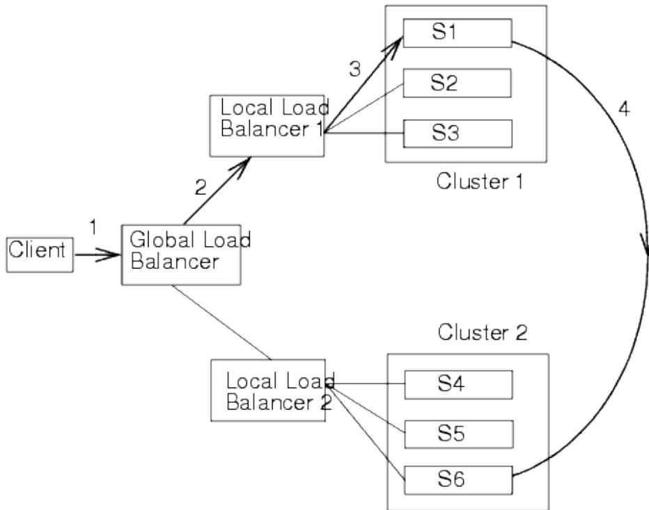
All Session state is sent synchronously from Server S1 to Server S6 in the remote cluster. If a custom replication channel was configured then all replication data is sent and received through that channel.
