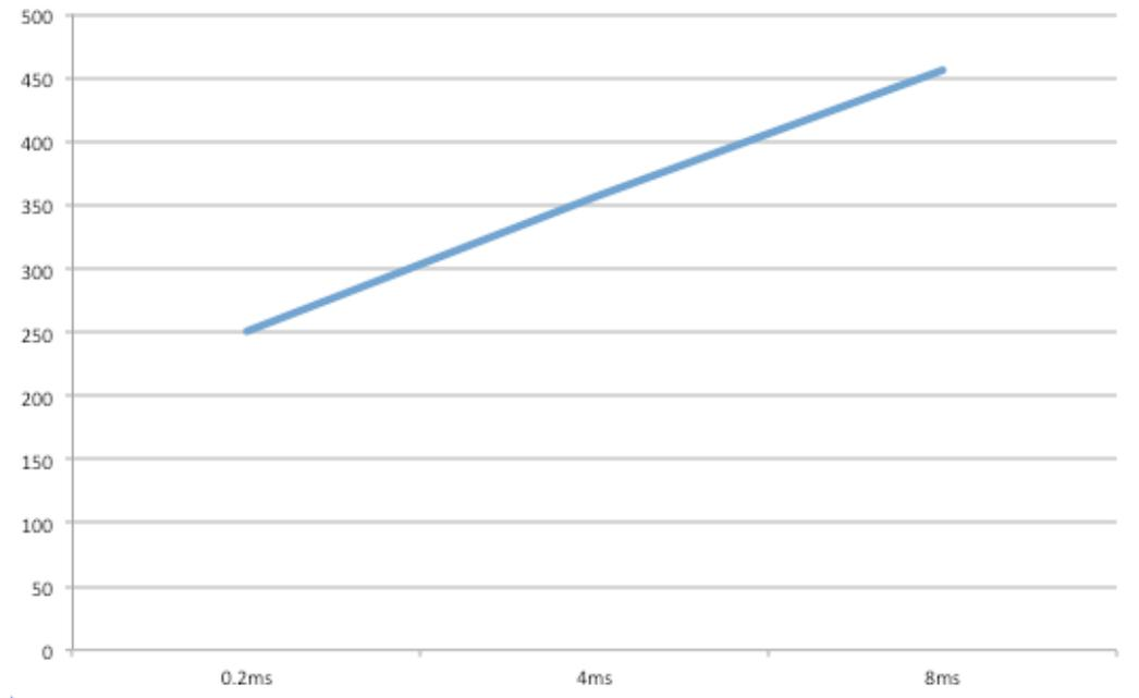
The vertical axis shows the User Response Time in milliseconds. The horizontal axis shows the measured RTT between the machine hosting the WebCenter Portal managed servers and the machine hosting the Oracle Database.
