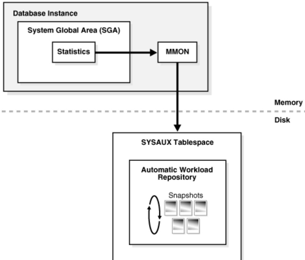
AWR can be configured to automatically collect performance statistical snapshots at regular intervals, or can be manually triggered. The ADDM utility can then be used to analyze the statistics between two snapshot intervals, to produce a performance summary report that includes:
