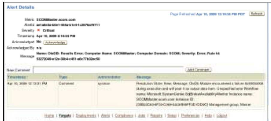
Figure 2. Shows a Microsoft SCOM alert message within the Oracle Enterprise Manager console.
