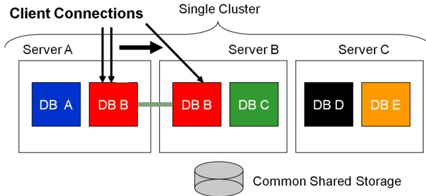
Online database relocation allows an online migration of a database from one server to another server. Online database relocation leverages the ability of Oracle Real Application Clusters to simultaneously run multiple instances servicing a single database.
