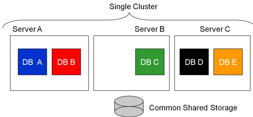
In this example configuration, we have five single-instance Oracle RAC One Node databases running in a cluster of three servers:
