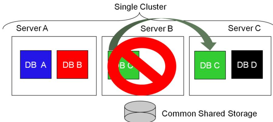
Oracle RAC One Node is integrated with Oracle Clusterware which monitors the health of the database and ensures database service availability. In the event of a failure, Oracle RAC One Node will detect the failure and either restart the failed database, or fail it over to another server.
