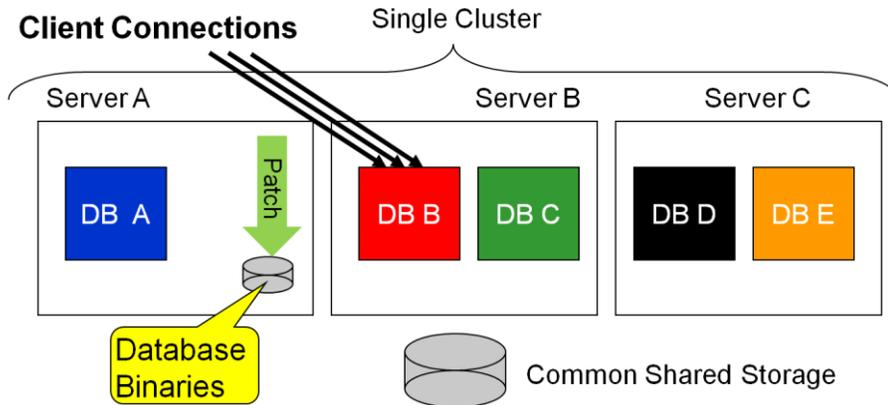
The figure above depicts a RAC One Node deployment after using online database relocation to move database B from server A to server B. After the migration, the database binaries that had hosted the instance formerly running on server A remain available for patching. Once patched, database B can be migrated via online database relocation back to server A.
