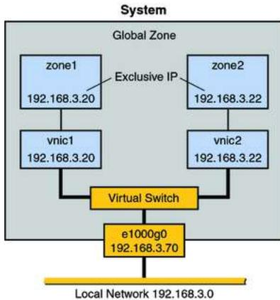
Figure 6. Oracle Solaris Zones enable VNICs (with unique hostnames and IP addresses) that are subject to resource controls.
