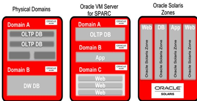
Figure 4. Zero-cost virtualization technologies are built into SPARC servers and Oracle Solaris.
