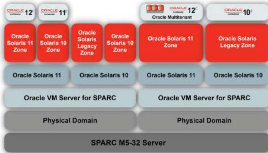
Figure 5. A hybrid approach can combine database and server-based consolidation approaches to optimize resource utilization, scalability, and management efficiency.
