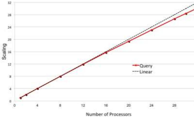
Figure 1. Oracle Solaris demonstrates near-linear scaling for data warehouse queries on Oracle's SPARC M5-32 server.
