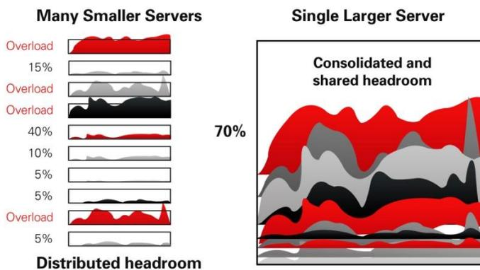
Figure 1. Consolidating and sharing headroom in large symmetric multiprocessing (SMP) servers.
