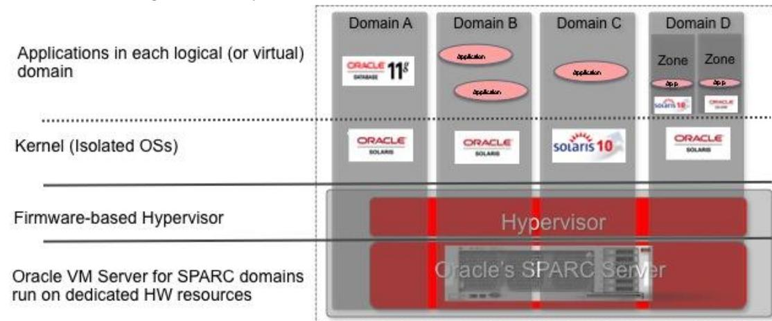
Figure 4. Oracle VM Server for SPARC virtualization.
