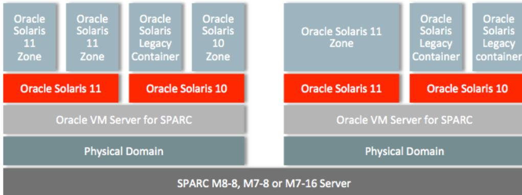
Figure 2. Virtualization technology stack on the SPARC M8-8, M7-8 and M7-16 servers.
