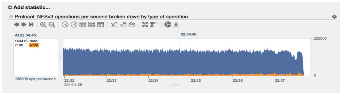
Figure 3. Oracle ZFS Storage Appliance ZS3-2 Analytics performance results of NFS protocol broken down by type of operation
