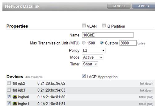
Figure 7. LACP, jumbo frame and MTU configurations on the Oracle ZFS Storage Appliance
