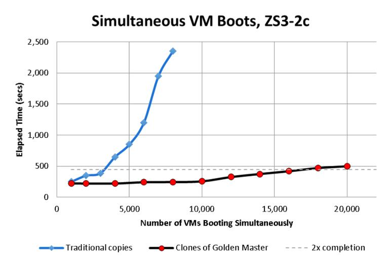
Figure 2. Simultaneous VMware virtual machines boot disks with Oracle ZFS Storage Appliance ZS3-2 (per head)
