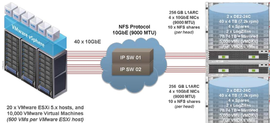
Figure 4. Oracle ZFS Storage Appliance – Disk layout for small virtual machines/virtual desktops with capacity disks for 10,000 VMware virtual machines
