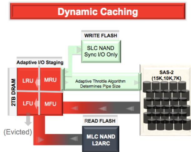
Figure 1. Dynamic caching functionality of the Oracle ZFS Storage Appliance
