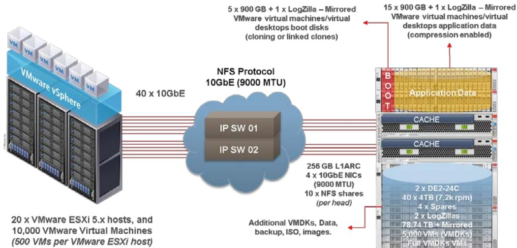
Figure 5. Oracle ZFS Storage Appliance – Disk layout for small virtual machines/virtual desktops with capacity disks for 10,000 VMware virtual machines
