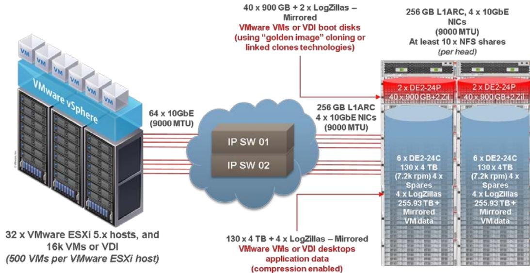
Figure 6. Oracle ZFS Storage Appliance – storage layout with capacity disks
