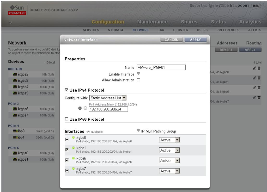
Figure 8. IPMP configuration on the Oracle ZFS Storage Appliance
