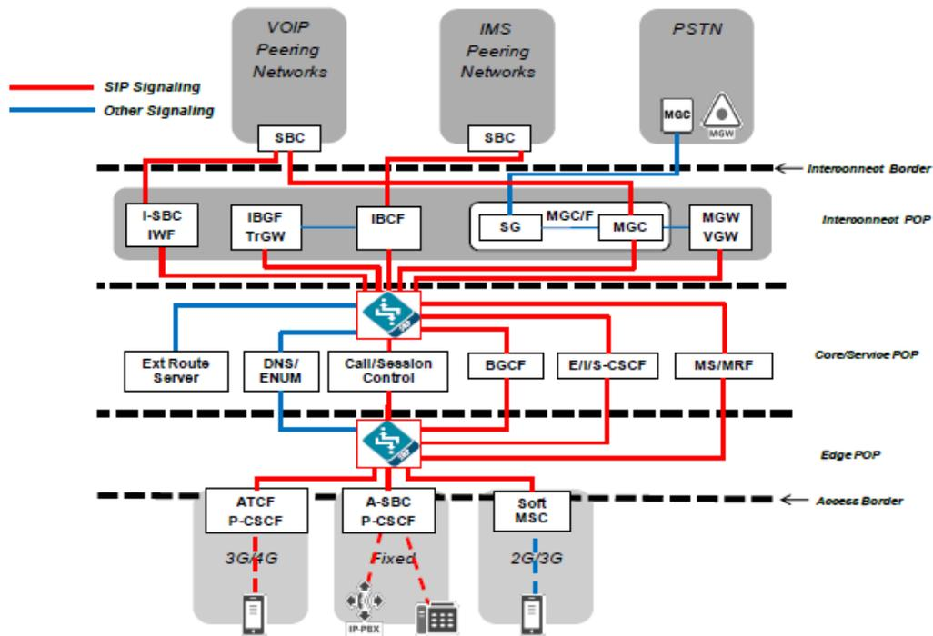
Figure 3: VoIP Interconnect and Peering Architecture Evolution
