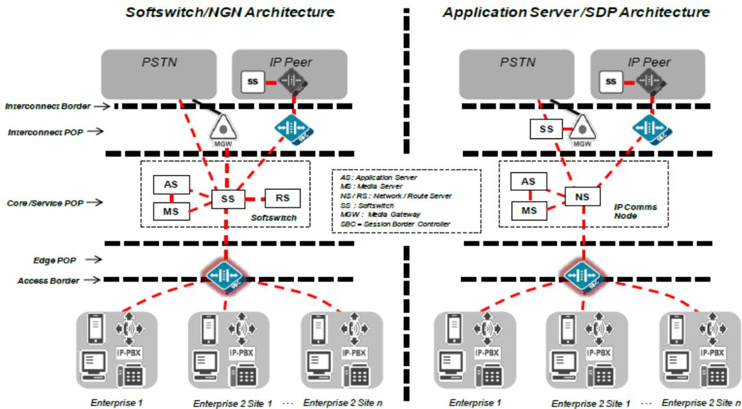
Figure 5: Enterprise VoIP/SBC Architecture
