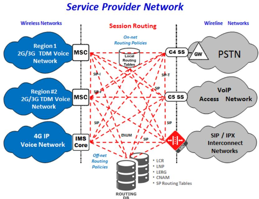
Figure 1: Signaling Core of Service Provider Networks
