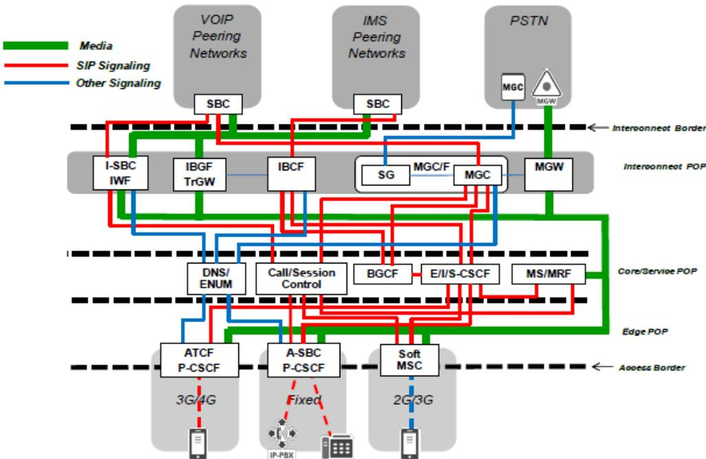
Figure 2: VoIP Interconnect and Peering Architecture
