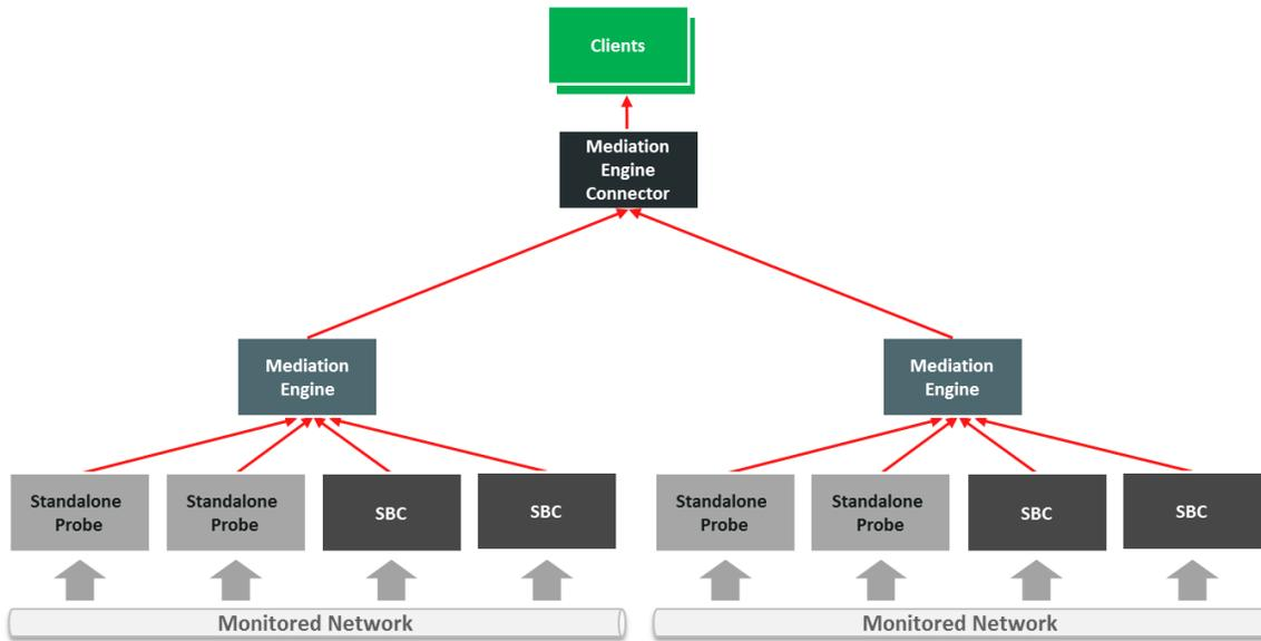
Figure 7: One OCOM System with 1 MEC, 2MEs, and Probes
