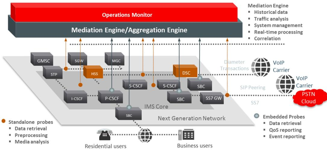
Figure 4: An Example of OCOM Deployment
