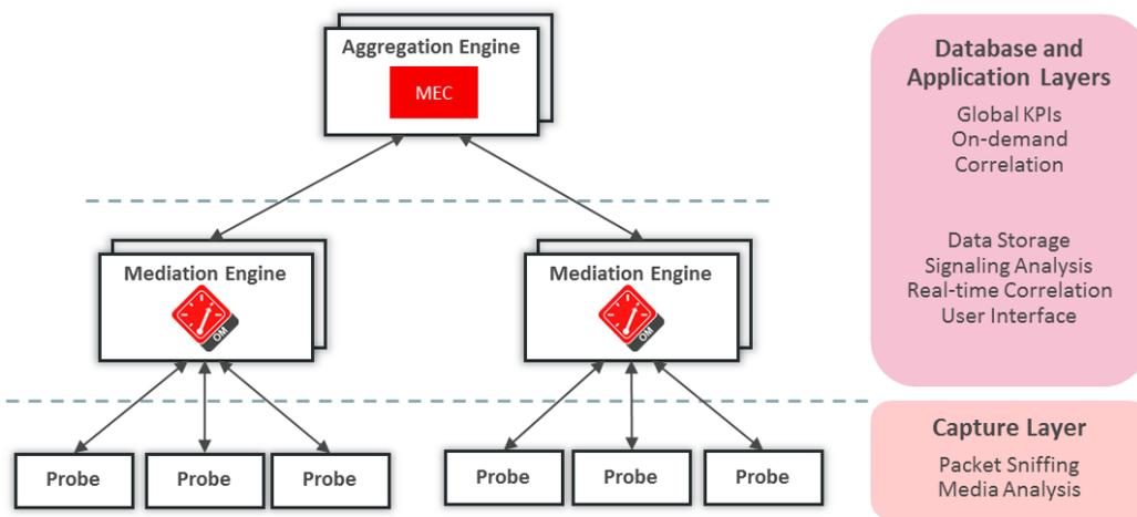
Figure 3: OCOM System Architecture
