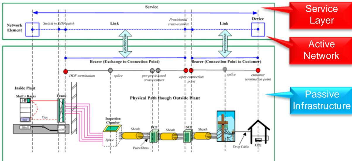
Figure 2 – Providing a “Service Ready” FTTx network with multiple layers
