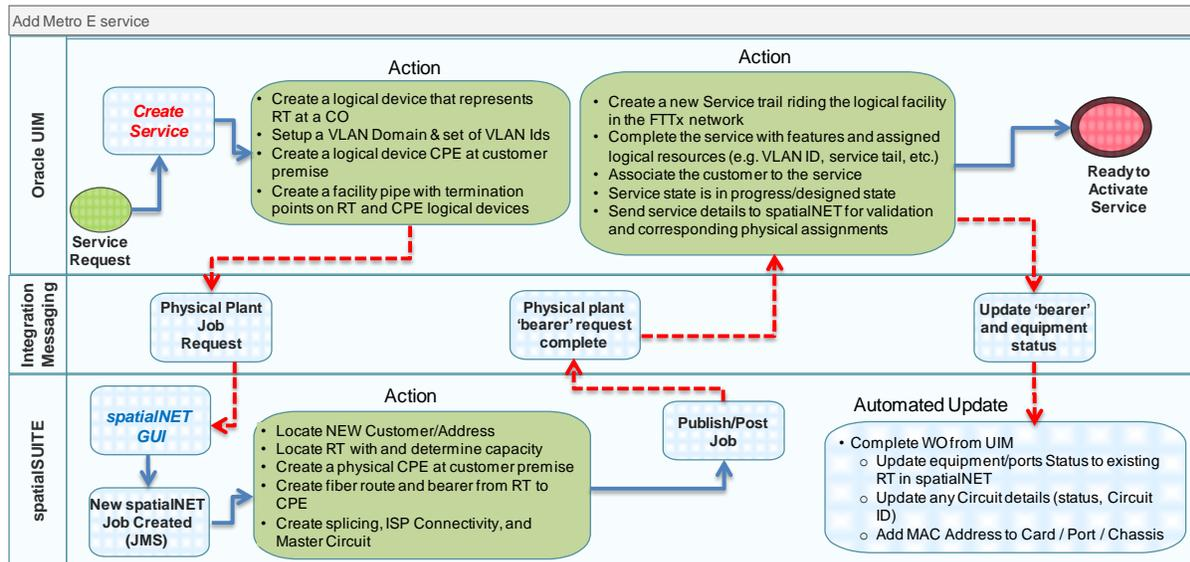
Figure 5 – Example Process Flow to Create Metro Ethernet Service over a FTTx Network
