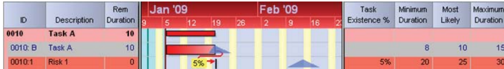
Figure 5. The project bar chart in Primavera Risk Analysis illustrates how the risk event delays the task.
