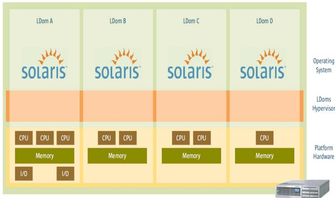
Figure 2. A single server hosts multiple domains, each running unique, isolated OS instances.
