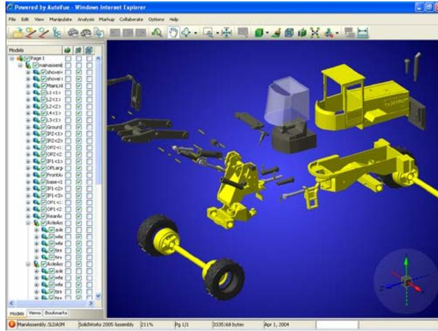
Figure 2: Explode 3D assemblies into component parts.
