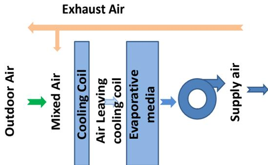
Figure 2: Schematic of air-handling unit
