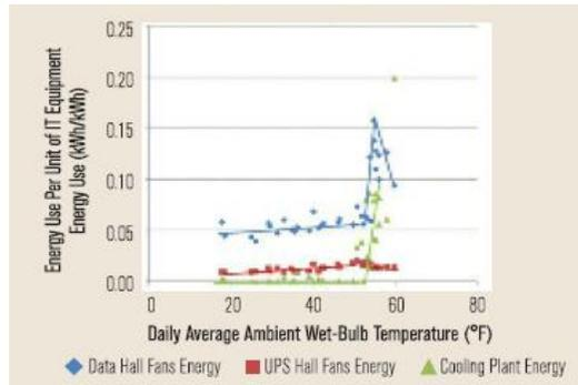
Figure 3: Cooling energy use vs. ambient wet-bulb temperature
