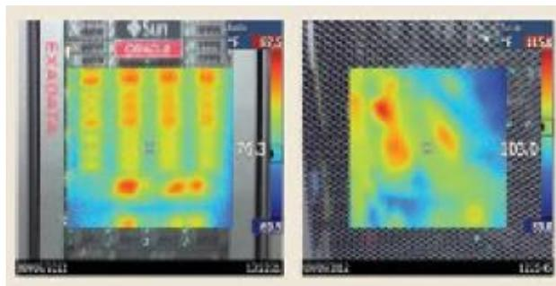
Figure 5: Thermograph of temperature profile at rack discharge
