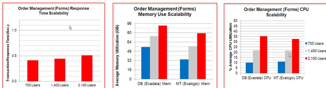
Figure 11: Response Time Scalability, CPU and Memory Scalability. Linear usage of memory and CPU.
