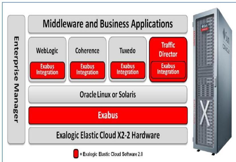
Figure 2: Key Software Components of Exalogic Elastic Cloud
