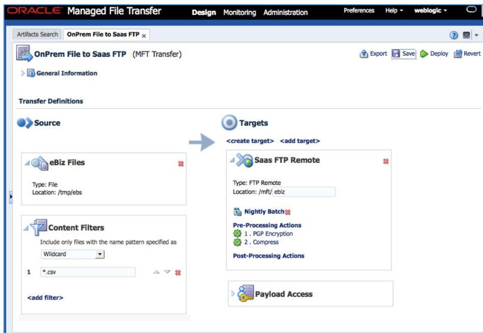
Figure 15: Oracle MFT On Premise to Cloud SaaS Transfer Example
