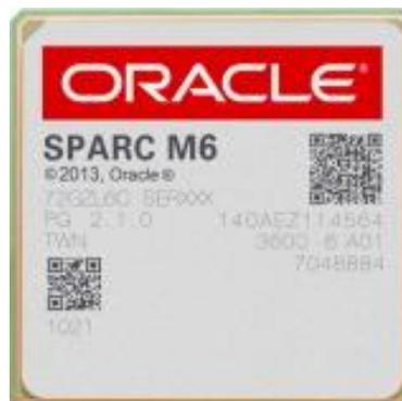
*Oracle's SPARC M6 processor is the industry's most scalable multi-thread, multi-core processor, delivering exceptional single thread performance and very high throughput while enabling systems with up to 96 sockets.*
