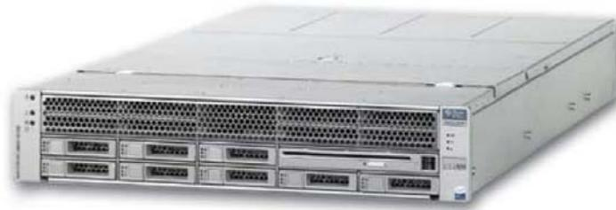
**The Sun Fire X4450 server can expand to up to 24 processing cores, 256 GB of memory, and more than 2 TB of internal storage.**
