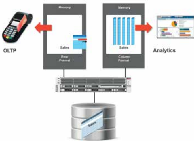
Figure 1: Oracle 12c– dual format in-memory database
