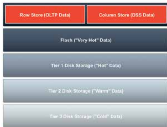
Figure 4: Oracle's multi-tiered database architecture
