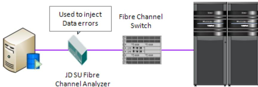
**Figure 2. Testing configuration**
