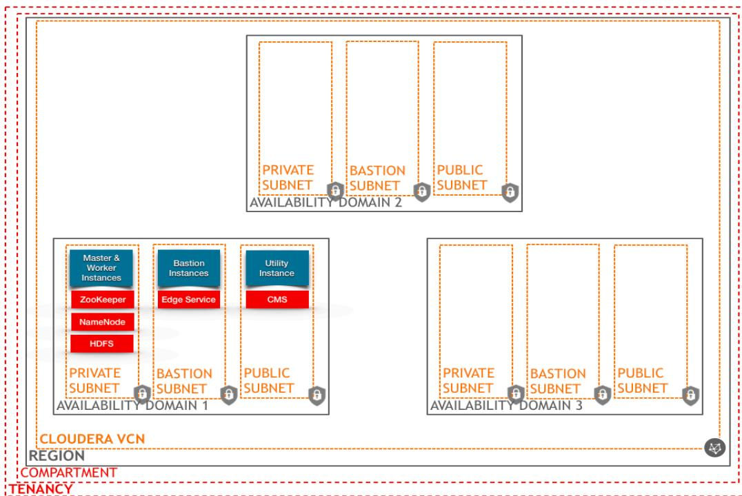
**Note:** It is also possible to install Enterprise Data Hub to span availability domains in a region, which allows for additional fault tolerance and high availability. Although this model is not currently supported in the automated Terraform deployment, Oracle plans to release availability-domain spanning templates to support this automated deployment model in the future. For more information, see “Availability Domain Spanning Deployment Model” in the Appendix.
