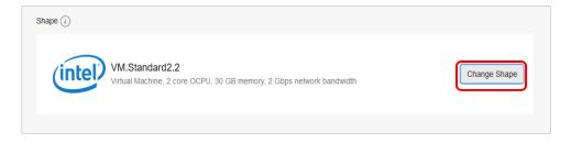
Select **Virtual Machine**, then select a shape. For the purposes of this lab, select either an Intel Skylake **VM.Standard2.2** shape, or under the Specialty and Legacy series, select the **VM.Standard.E2.2** shape.
