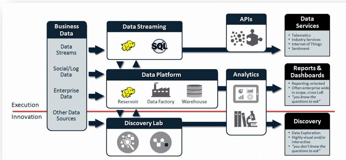
**FIGURE 1: 4TH GENERATION DATA ARCHITECTURE FOR BIG DATA IS EMPHASIZES INTEGRATION WITH CRUCIAL DATA REQUIREMENTS INCLUDING DATA STREAMING, DISCOVERY, ENRICHMENT, TRANSFORMATION AND GOVERNANCE.**
