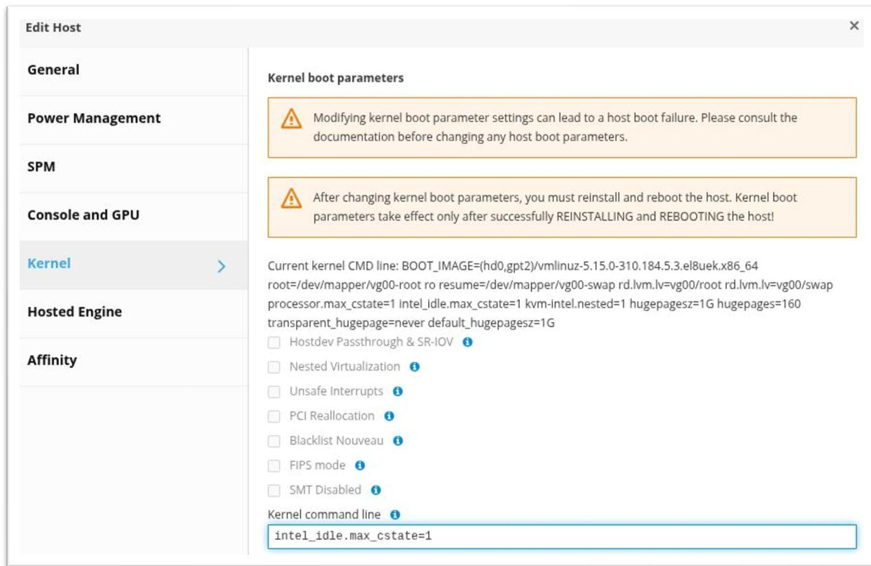
Complement the OS settings with firmware controls. Select a Maximum Performance power profile and, if necessary, disable deep package C-states and C1E while keeping turbo and P-states enabled unless instability is observed. Avoid extreme options such as `idle=poll`, which dramatically increase power consumption and thermals.
