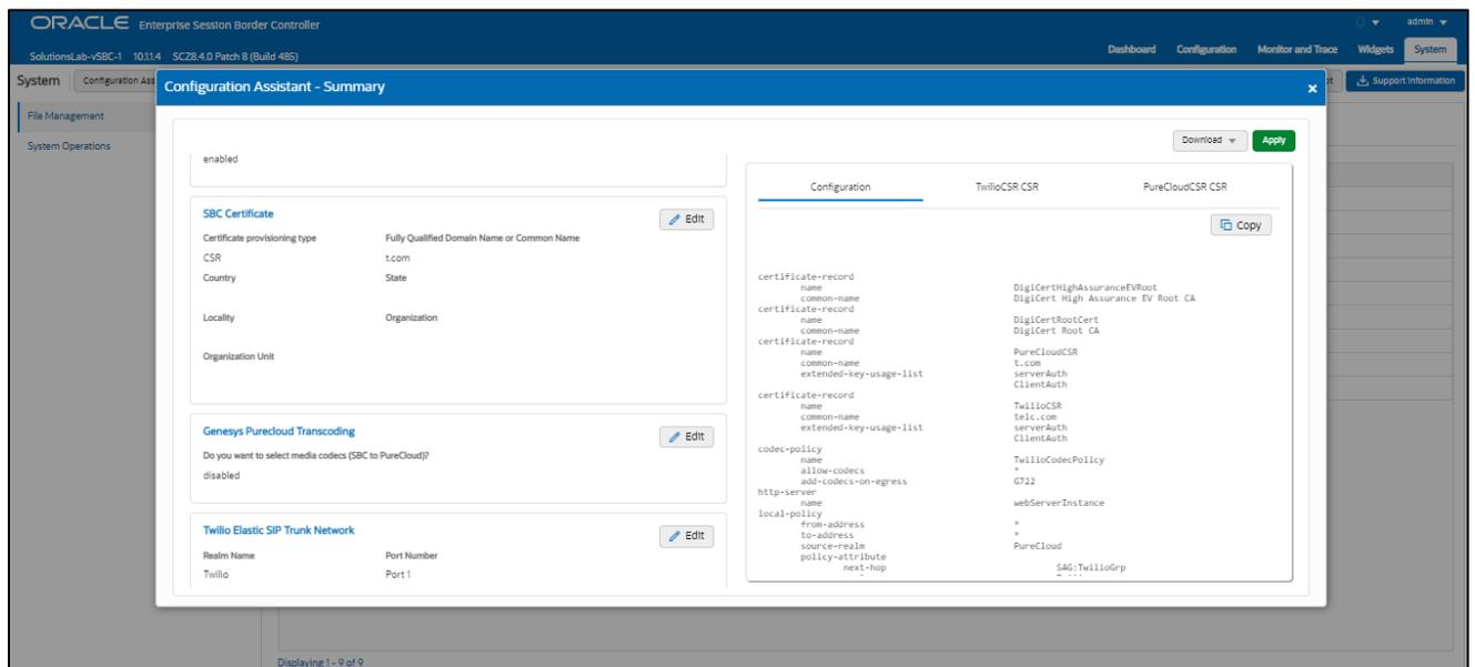
Click the copy button under the CSR and paste the output into a text file. Next, provide the txt file to your CA for signature. Once the certificate is signed by the CA, you will need to import that certificate into the SBC manually, either via ACLI or through the GUI.
