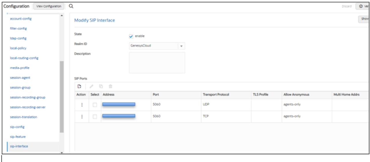
Once sip-interface is configured – the SBC is ready to accept traffic on the allocated IP address.
