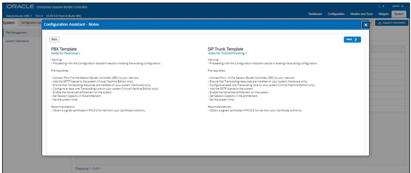
Clicking “Next” on the Notes page triggers the configuration assistant to do a system check. This ensures that all of the system requirements for the platform and sip trunk you have selected have been met before proceeding to configuration pages. If they have not been met, you will be greeted by a page providing the opportunity to setup entitlements, add license keys, etc. before moving on to the configuration.
