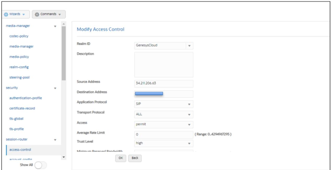
Notice the trust level on this ACL is set to high. When the trust level on an ACL is set to the same value of as the access control trust level of its associated realm, this create an implicit deny, so only traffic from IP addresses configured as ACL's with the same trust level will be allowed to send traffic to the SBC. For more information about trust level on ACL's and Realms, please see the [SBC Security Guide, Page 3-10](#).
