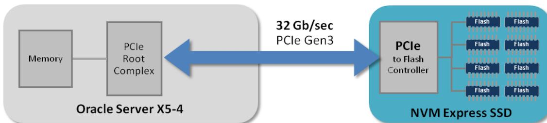
Figure 3. Oracle NVMe solid state drive architecture
