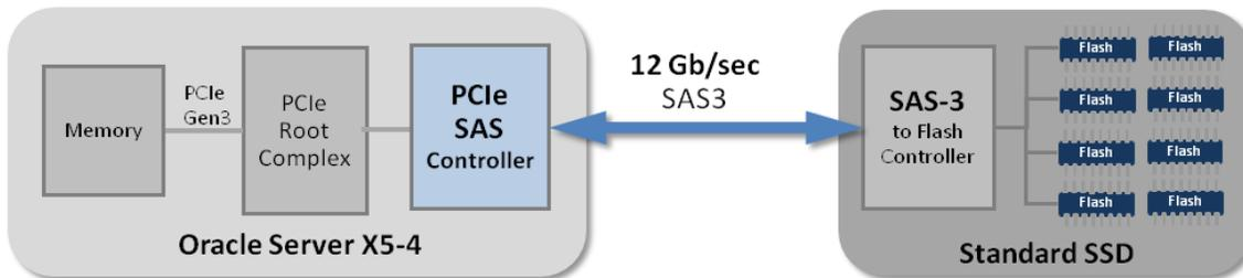
Figure 2. Traditional SAS-3 solid state drive architecture
