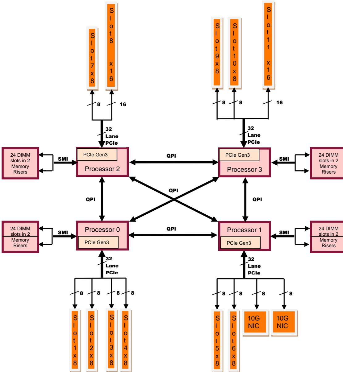
Figure 4. Oracle Server X5-4 system design
