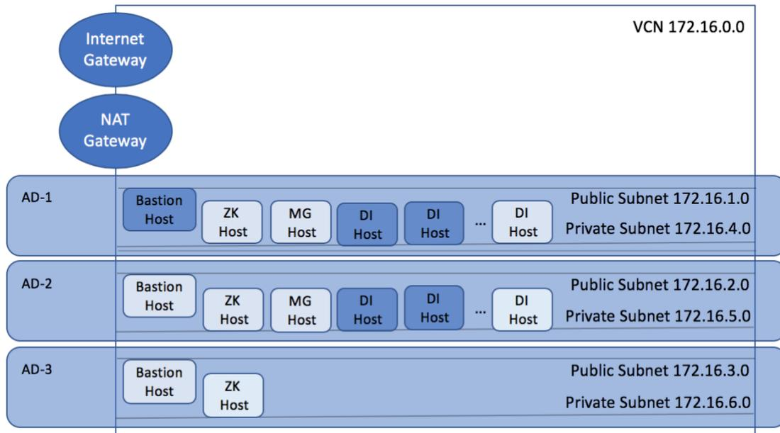
**Oracle TimesTen Scaleout Deployment Possibilities.** Dark shading indicates default host deployment.
