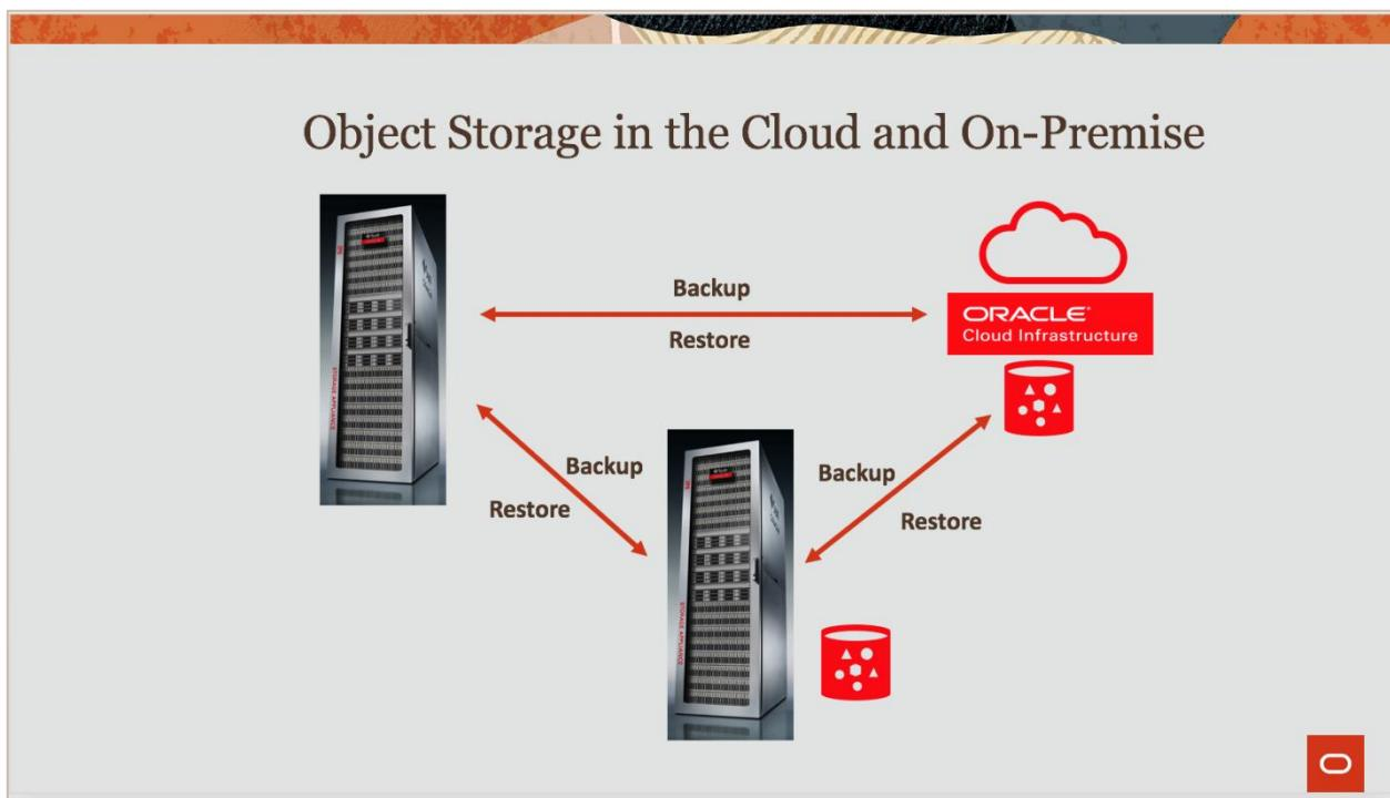
The ZFS Appliance on the left takes on the role of the source from which shares and LUNs can be exposed to clients. The source can initiate a snapshot and then send that snapshot to the target ZFS Appliance, which is another node<sup>1</sup> over a defined network.
