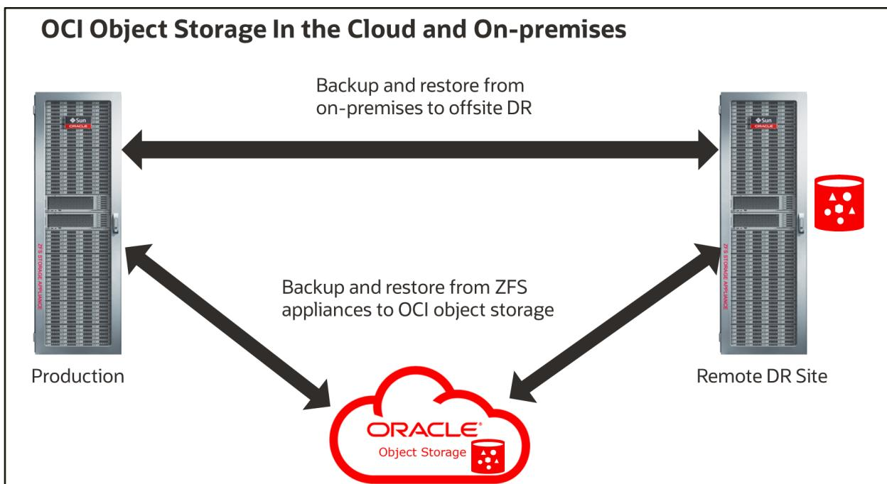
The ZFS Appliance on the left takes on the role of the source from which shares and LUNs can be exposed to clients. The source can initiate a snapshot and then send that snapshot to the target ZFS Appliance shown on the right, which is another node over a defined network, or it may send the snapshot directly to object storage in OCI.
