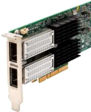
*The Oracle Dual Port QDR InfiniBand Adapter M3, a part of Oracle’s InfiniBand and network virtualization portfolios, is designed to provide maximum fabric bandwidth to servers and storage supporting PCI Express® 3.0. The Oracle Dual Port QDR InfiniBand Adapter M3 enables applications to take full advantage of the I/O capabilities integrated into Oracle’s latest servers, doubling the network bandwidth available in high-performance application and server virtualization environments.*
