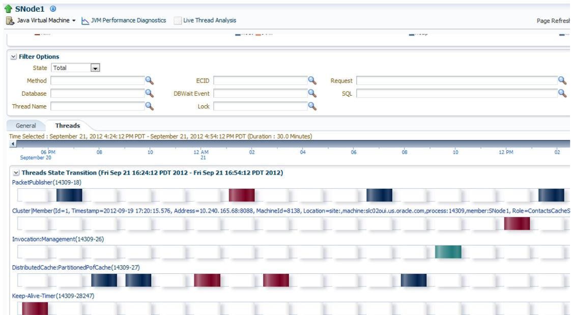
Figure 9 – Thread state transition and ability to search threads by state (DB wait, IO wait, etc)
