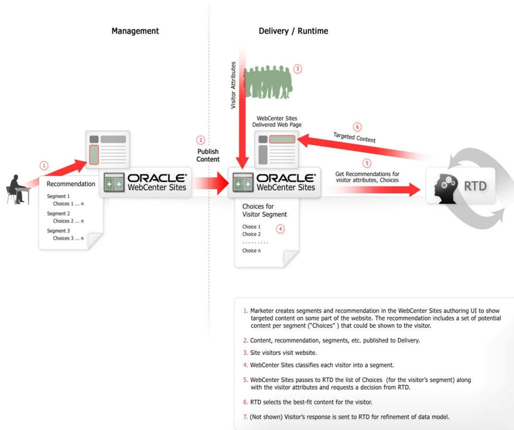
Figure 8: WebCenter Sites and RTD: Controlled Automation – Marketer does first-level segmentation in WebCenter Sites
