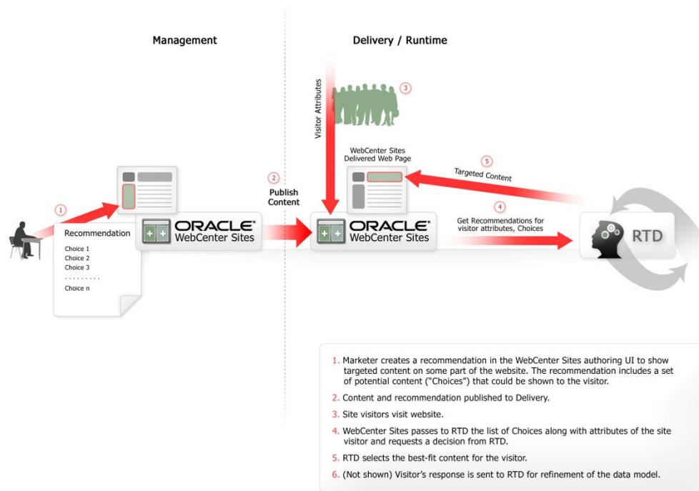
Figure 5: WebCenter Sites and RTD: Full Automation – RTD manages all customer segmentation
