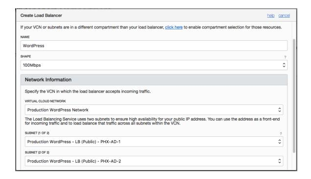
The load balancer shape will determine the amount of traffic the load balancer can handle (100Mbps, 400Mpbs, or 8000Mpbs).
