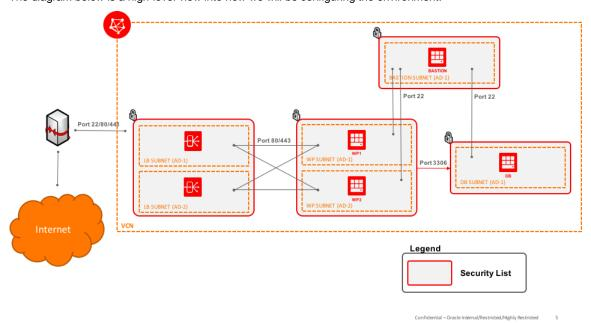
In this white paper we will set up a VCN across multiple Availability Domains (AD), set up a bastion host to allow for access to the environment from the Internet, set up the application tier for WordPress across two ADs, set up the database tier for WordPress, configure the WordPress application, set up the load balancer to front end the WordPress application and load balancing are functioning as expected.
