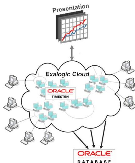
TimesTen In-Memory Cache Grid was configured on all 8 compute nodes in the Exalogic machine. Four cache grid members were configured for each compute node to take advantage of the compute power and available RAM.
