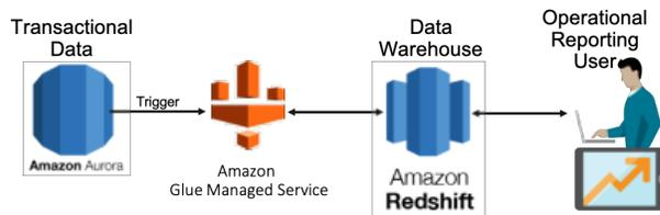
From the data catalog the ETL engine enables the DBA to create an ETL job by selecting the source and target data stores from the AWS Glue data catalog. Target schemas are provided by the data catalog. Then the DBA defines the ETL job where upon Glue generates PySpark code, which often needs to be customized based on validation and transformation requirements.
