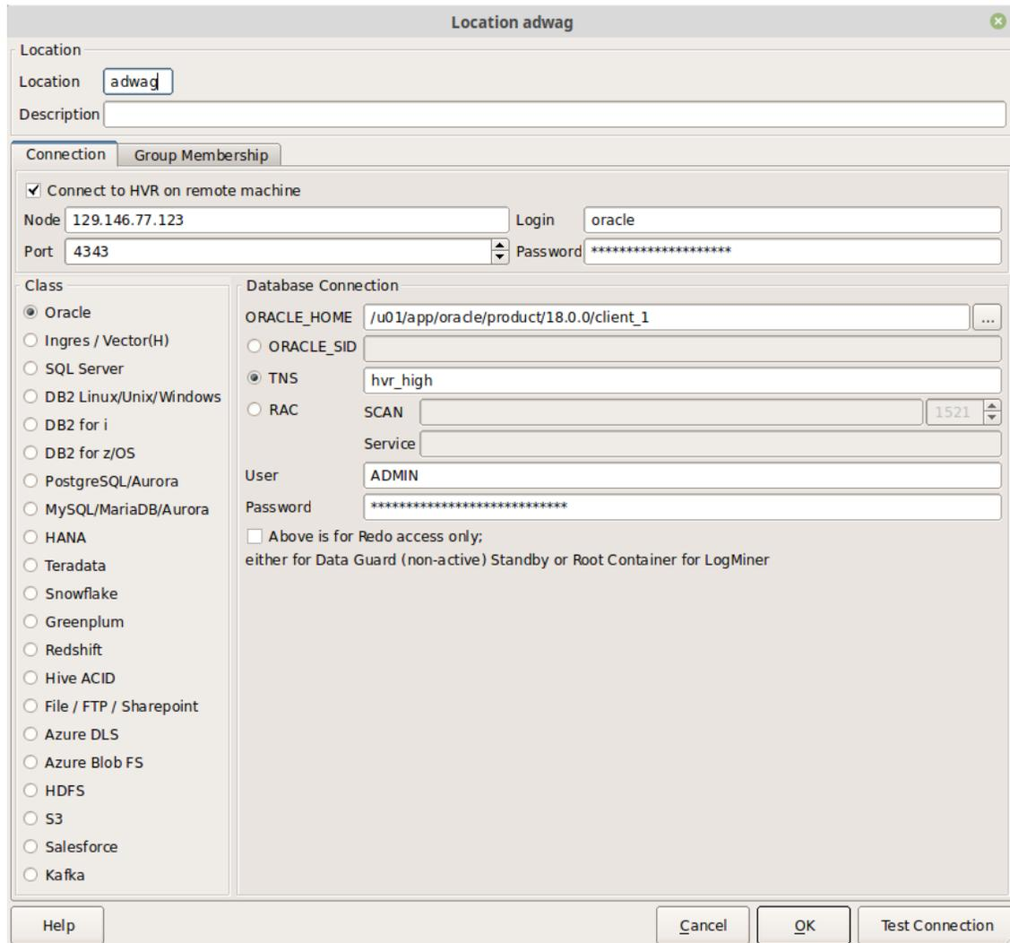
Figure 3. Connecting to Oracle ADWC through an agent.
