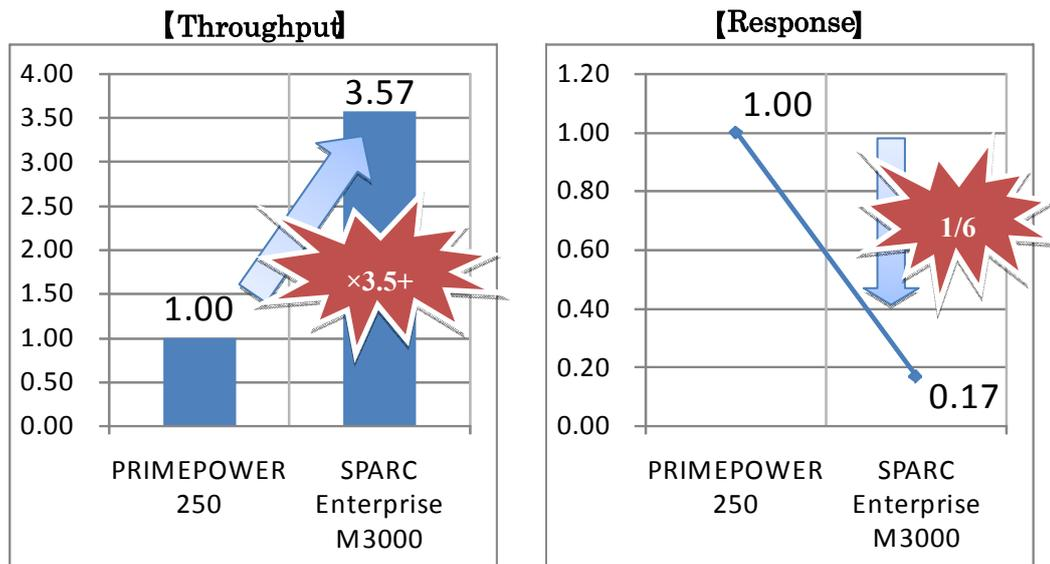
**Figure 3-1 Performance comparison of PRIMEPOWER 250 and SPARC Enterprise M3000**
