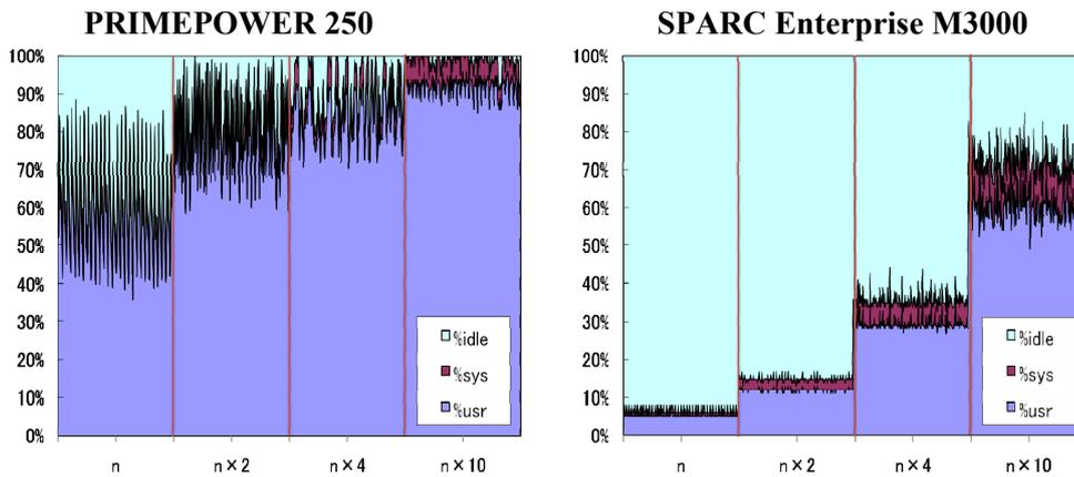
Figure 6-6 Changes in CPU usage by multiplicity
