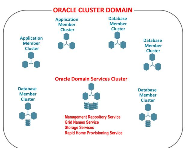
**Oracle Cluster Domain Database Database Database Application Member Cluster Member Cluster Member Cluster Member Cluster Uses IO & ASM Uses ASM** Uses local ASM GI only Service Service of DSC **Oracle Domain Services Cluster** Mgmt Rapid Home Provisioning **Additional** ACFS **ASM ASM** Repository **Optional** (GIMR) (RHP) Services Service **IO Service** Services Service Service **Shared ASM**
