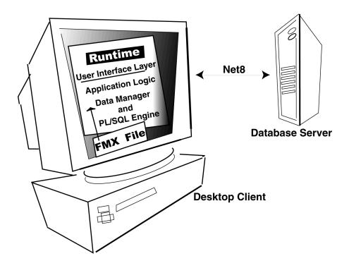
Figure 15–1 Legacy Forms Server client-server-based architecture
