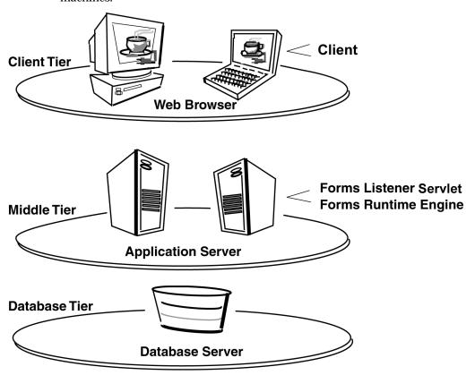
Figure 15–2 Forms Services Web-based architecture
