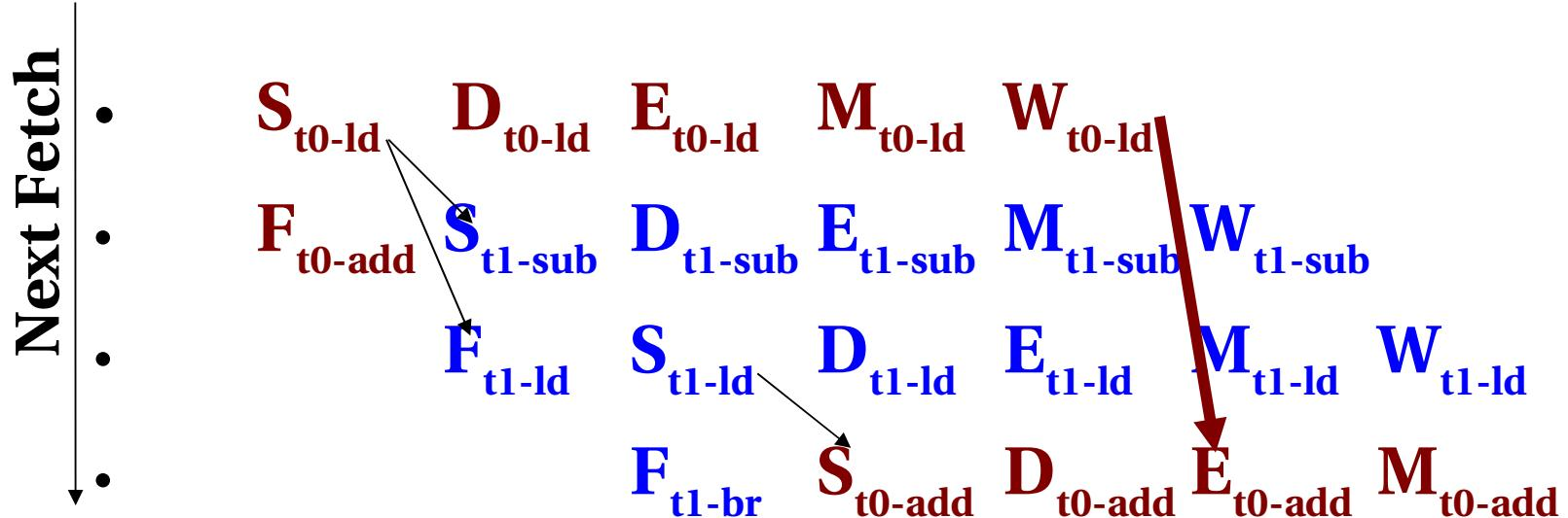
Thread '0' is speculatively switched in before cache hit information is available, in time for the 'load' to bypass data to the 'add'
