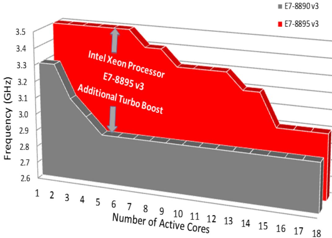
Figure 9. Comparison of Intel Xeon E7-8895 v3 processor to Intel Xeon E7-8890 v3 processor
