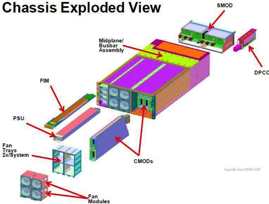
Figure 11. Chassis exploded view
