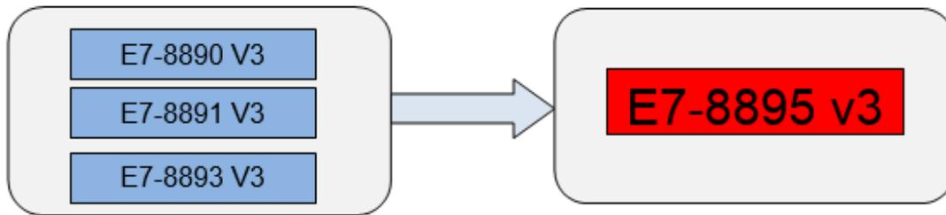
Figure 8. Elastic computing with a single processor SKU
