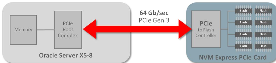
Figure 5. Oracle's NVMe SSD architecture
