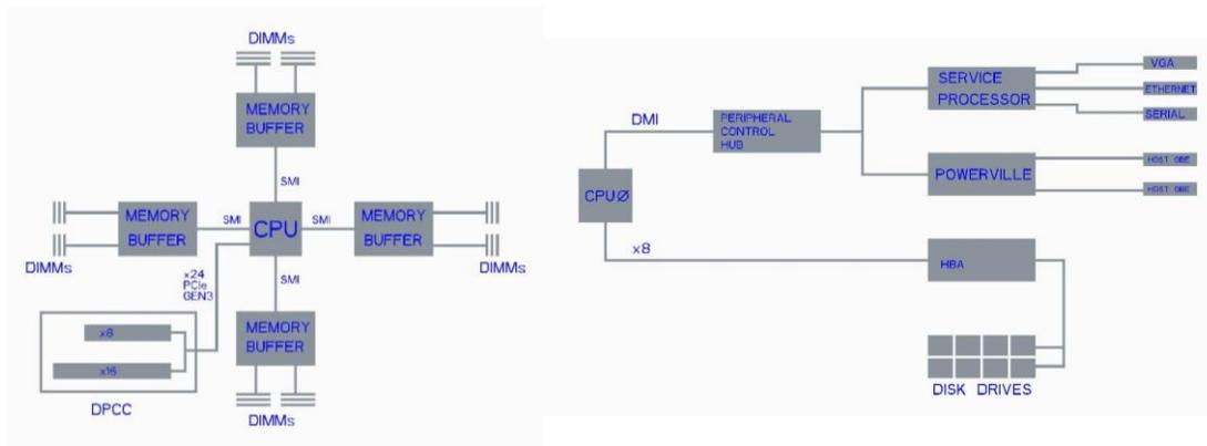
Figure 10. Oracle Server X5-8 System Block Diagram
