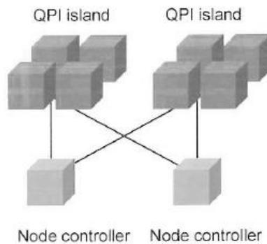
Figure 7. Glued architecture
